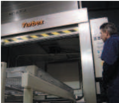
It is usual for multi-stage aqueous systems to include washing and rinsing processes, and sometimes hot air drying after the final rinse, says Turbex
