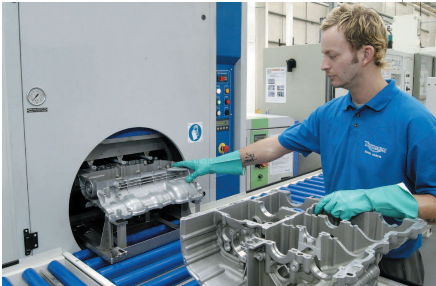
Birmingham-based Hydraforce is using MecWash aqueous washing machines featuring ultrasonics as part of the cleaning process for complex hydraulic valves – six separate component designs are cleaned including a new transmission manifold
