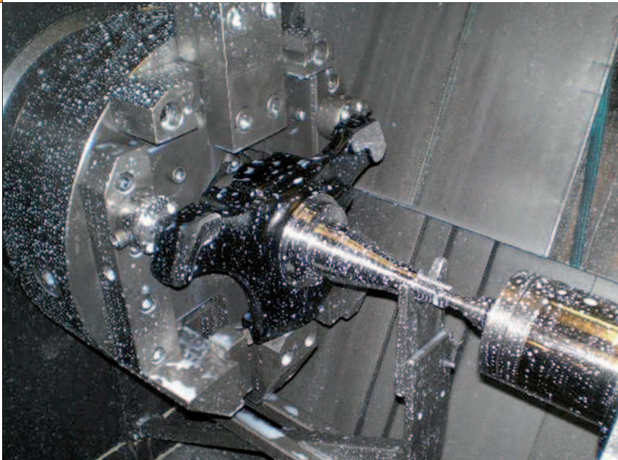
Machining axle components at Albion Automotive with the help of TaeguTec tooling
