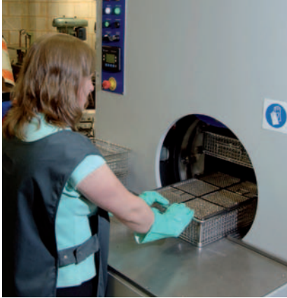
Rowan Precision says its aqueous degreasing system can better solvent cleaning results
