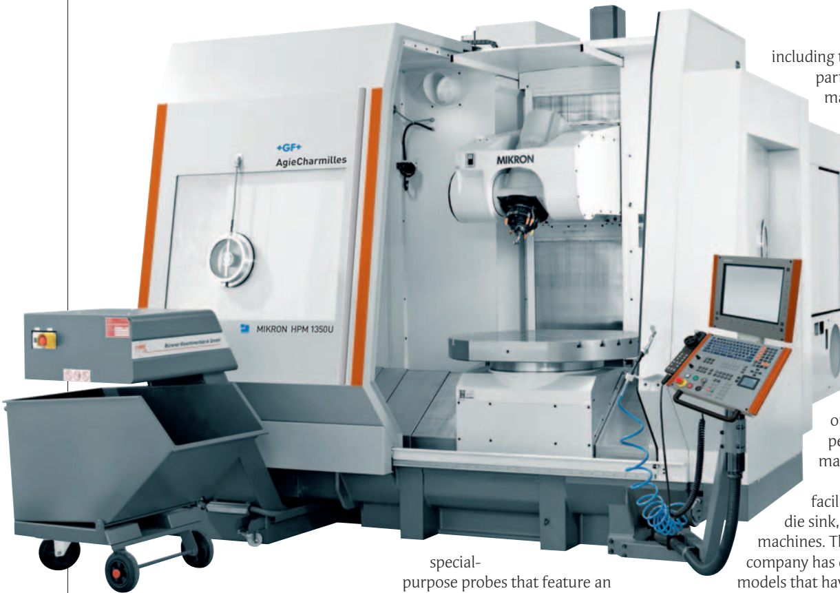
Arden Precision has installed its second Mikron 5-axis machining centre. Cycle times have been reduced by up to 30 per cent
