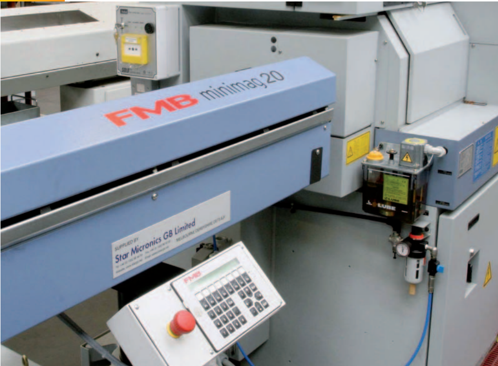
The new FMB Minimag 20 can feed 20 mm diameter bar without the need for end preparation
