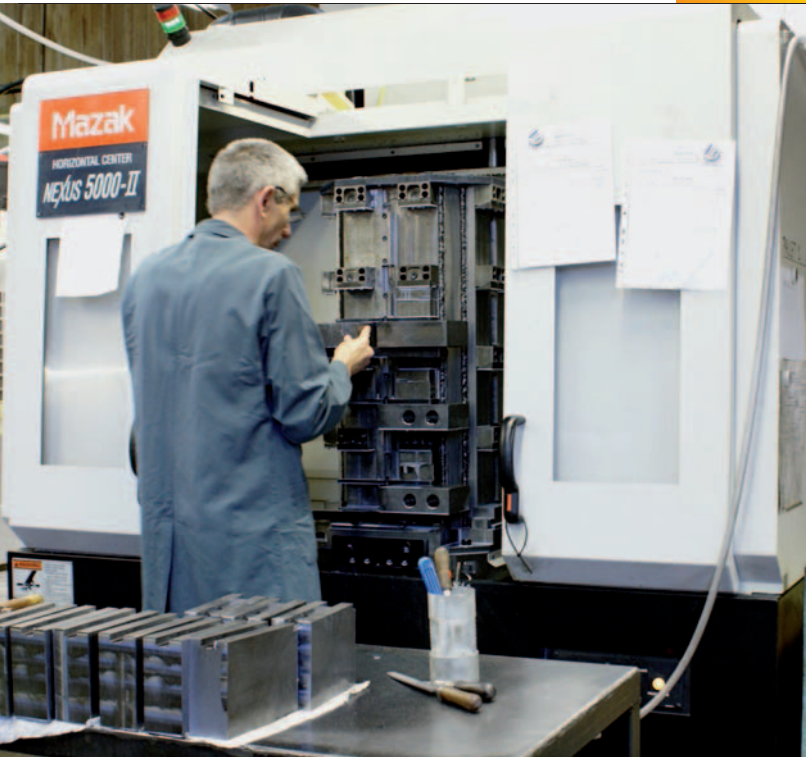
Thame Workholding installed two Mazak Nexus 5000-II horizontals following reliable performance from a previous horizontal from the same company
