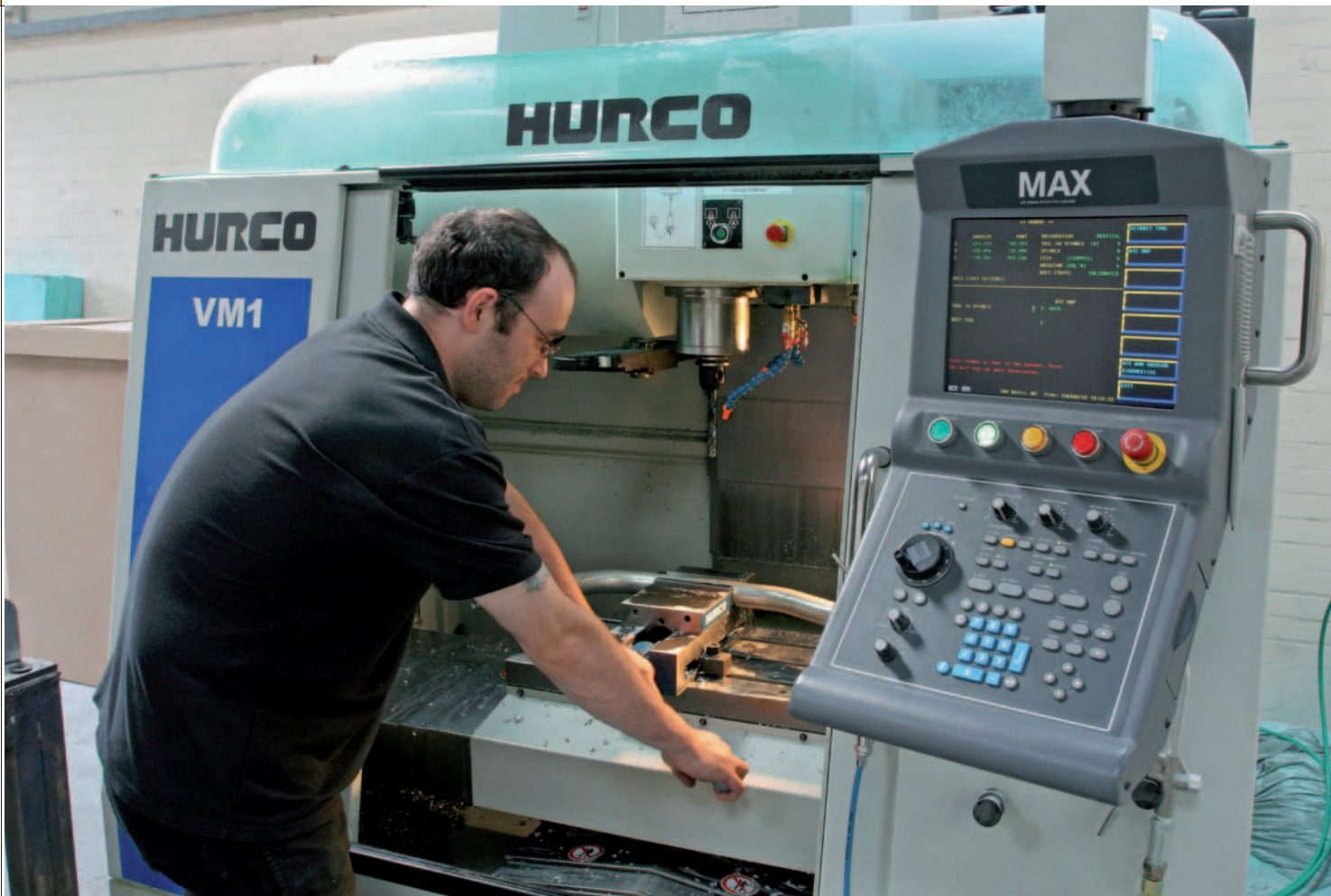
BFO's Steve Atkins is a designer not a CNC programmer, so the Hurco's Max CNC makes it easy for him to construct programs conversationally
