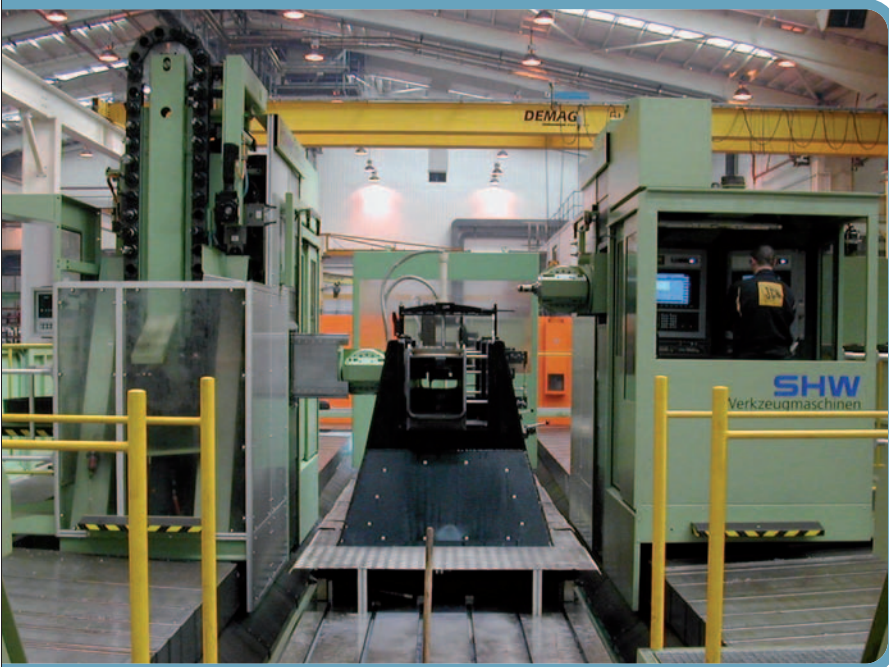
Machining both sides of a boom at once at JCB on a SHW Powerspeed 5 Duplex machine
