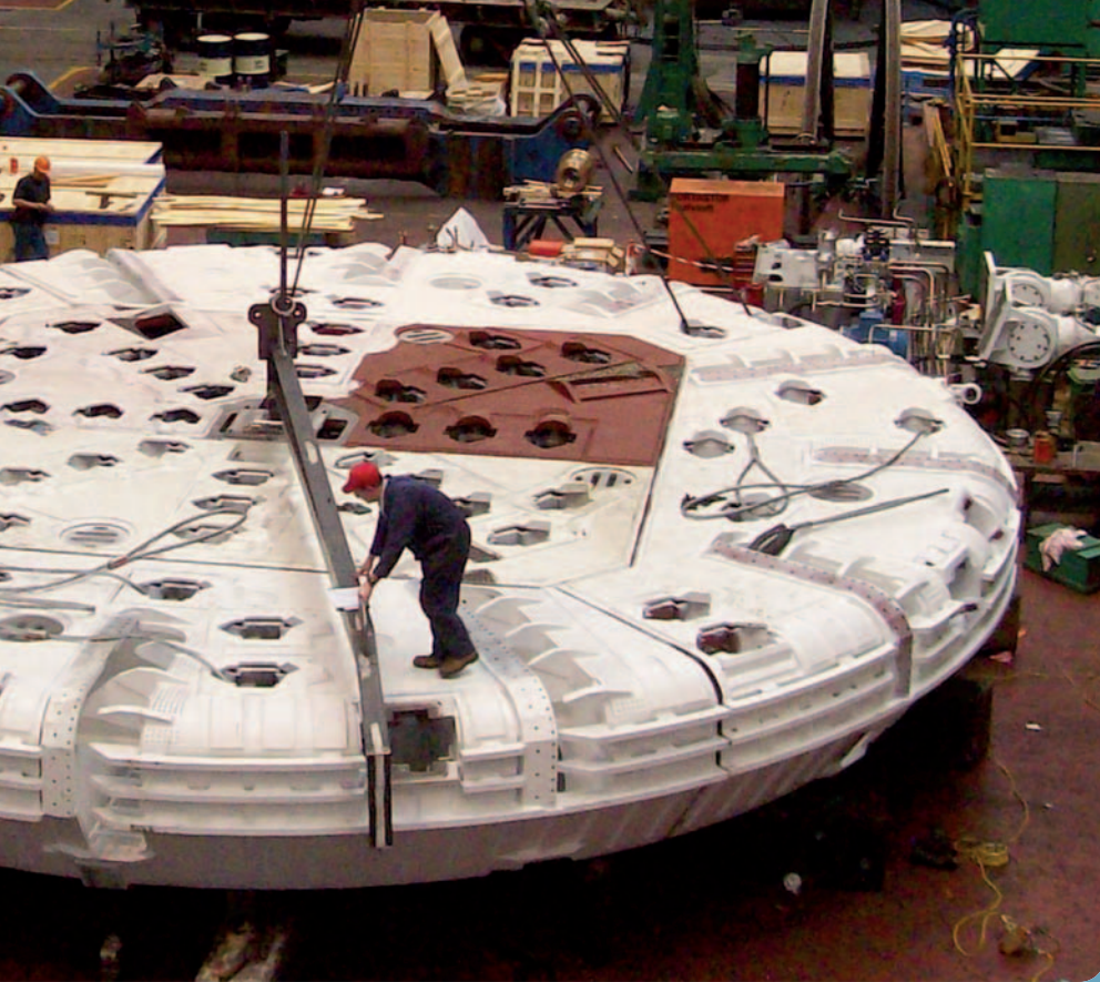
Destined for China; made in Sheffield. A 320 tonne boring machine head
