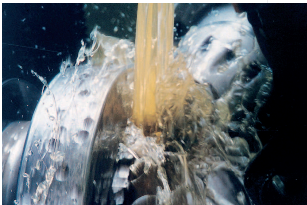
Fuchs' Ecocool Ultralife water-soluble coolants prevent bacteria proliferation
