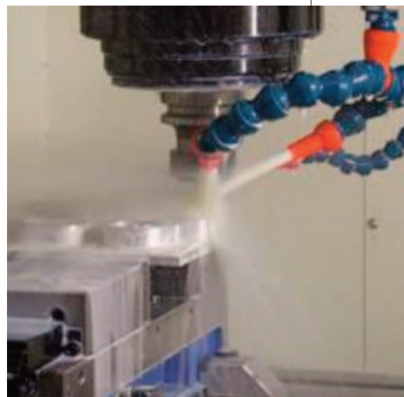
All-Cool 3000, a low-oil emulsion with low levels of bacterial control agents
